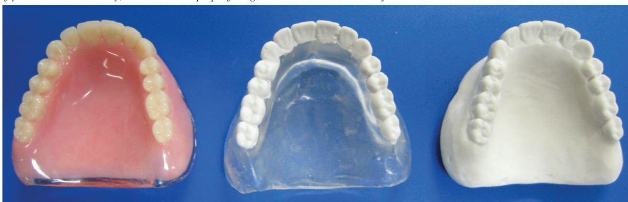
Figure 30. Denture and two different types of guides. The middle one uses clear acrylic for the base and Lang Dental's JET XR for teeth. The one on the right uses Lang Dental's JET XR 40% for the teeth area (opaque) and 20% for the base (Shadow).
