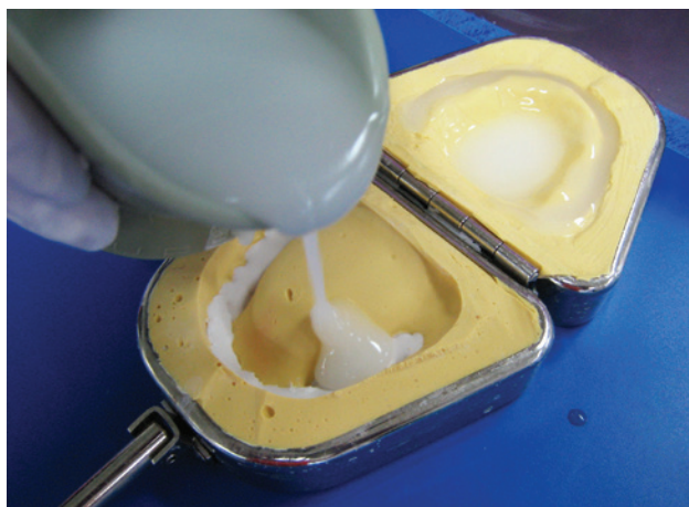
Figure 20. Mix clear acrylic and pour into both sides of mould.
