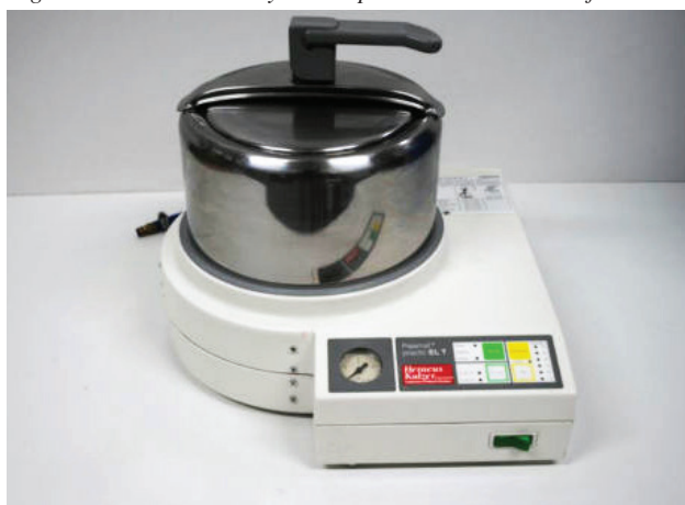
Figure 22. Cure the acrylic for 15-20 minutes in a warm pressure pot. Don't make it too hot!
